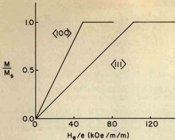
FIG. 6. Magnetization curves for the  $\langle 100 \rangle$  and the  $\langle 111 \rangle$  problem in YIG.
