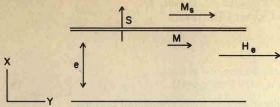
FIG. 1. Geometry for shock-induced demagnetization. Infinite half-space of ferromagnetic material in region  $x > 0$ . Uniaxial strain in region behind the shock  $S$ . Applied field  $H_e$  in transverse direction. Reduction in magnetization occurs across the shock front.
